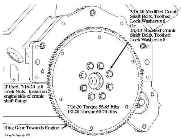
CAREFULLY ALIGN THE HUB SPACER/FLEX PLATE AND THE CRANKSHAFT BOLT HOLES WHILE PLACING THE HUB SPACER ONTO THE CRANKSHAFT. THE HUB SPACER SHOULD BE A CLOSE FIT TO THE CRANKSHAFT. INSTALL THE CRANKSHAFT BOLTS & NUTS AND TORQUE TO THE PROPER VALUE.
