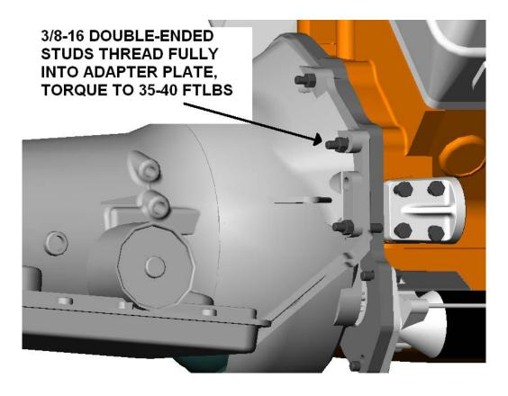
THREAD THE DOUBLE ENDED STUDS FULLY INTO THE ADAPTER PLATE USING THREAD LOCKING COMPOUND BEFORE INSTALLING TRANSMISSION
