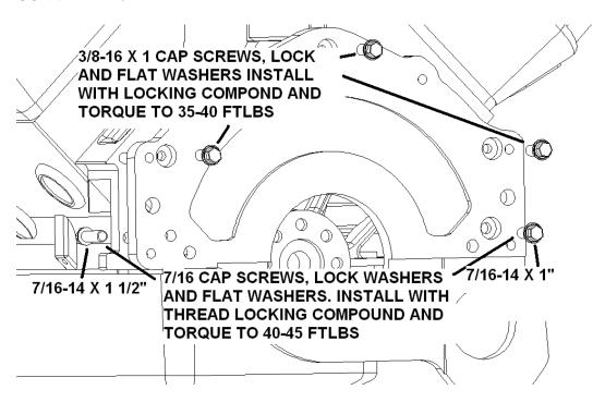
USING THE SUPPLIED BOLTS, BOLT THE ADAPTER PLATE TO THE BLOCK. IF NECESSARY USE A RUBBER MALLET TO FIT THE PLATE UP TO THE BLOCK FLUSH. DO NOT USE THE BOLTS TO FORCE THE PLATE ONTO THE BLOCK. THE PLATE SHOULD FIT FLAT TO THE ENGINE BLOCK WITH NO ROCKING OR GAP.
