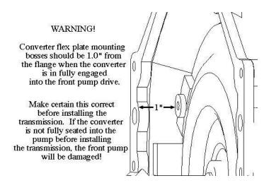
CHECK THAT THE CONVERTER IS SEATED INTO THE FRONT PUMP PRIOR TO INSTALLING THE TRANSMISSION. CHECK THE "PULLBACK" DISTANCE OF THE CONVERTER PRIOR TO INSTALLING THE CONVERTER TO FLEX PLATE BOLTS.
