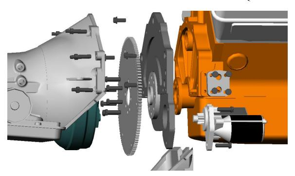
CLEAN THE CRANKSHAFT HUB, BACK OF THE BLOCK, FRONT OF THE TRANSMISSION BELL HOUSING AND THE TOROUE CONVERTER HUB OR
